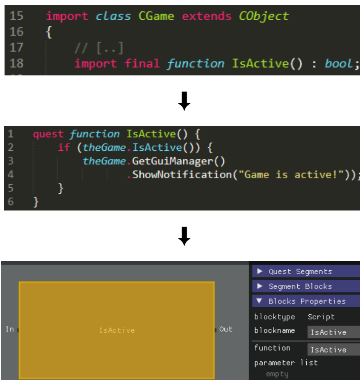
Illustration 31: Screenshots of one way how REDscript blends into the abstraction hierarchy: by exposing C++ engine/ game features and building on them for use in the next higher level.
