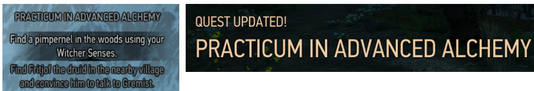
Illustration 19: Screenshots showing how the questgraph state is communicated via the in-game HUD. The left screenshot shows the current quest's objectives and the focused objective, the right shows a pop-up when a description or objective has been updated.
